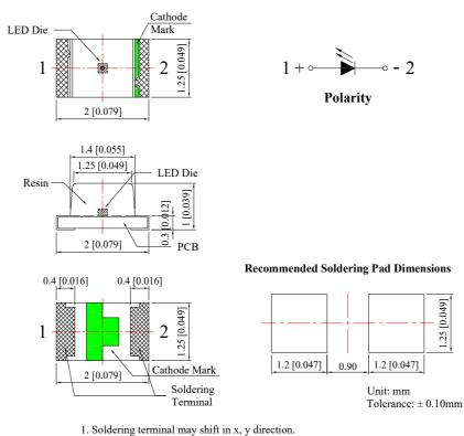
2. Polarity referring onto the cathode mark is reversed on the UR/HR/SR.
