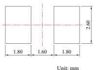
Unit: mm Tolerance: ± 0.10mm
