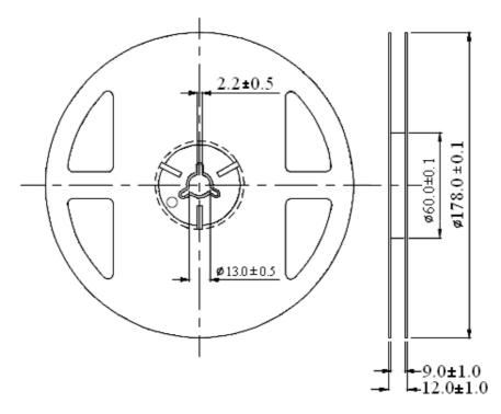
Unit: mm Tolerance:  $\pm 0.25$ mm
