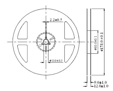
Unit: mm Tolerance:  $\pm 0.25$ mm
